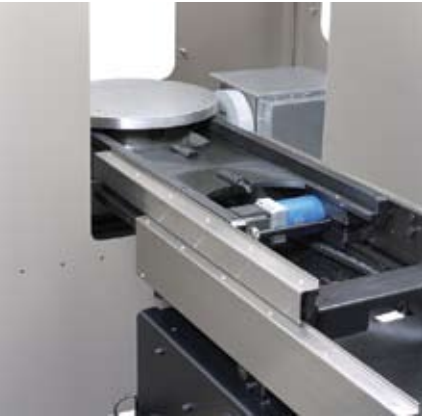
Linear guided pallet delivery system is shown loading pallet onto receiver.
